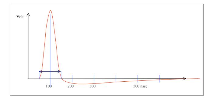
All observations in testbeams later on were in good agreement with these TileCal specifications, where obvously ,hard differentiation' was built-in. High rates could not be observed in testbeams.
