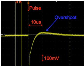
Using the baseline before the pulse as a reference At 10us  $\rightarrow \Delta V \sim 40 \text{mV}$ At 30us  $\rightarrow \Delta V \sim 0 \text{mV}$ Exists even at the lower charges. For 50 pC per PMT At 10us  $\rightarrow \Delta V \sim 3 \text{mV}$ At 30us  $\rightarrow \Delta V \sim 0 \text{mV}$  $\Delta t 30 \text{us} \rightarrow \Delta V \sim 0 \text{mV}$
